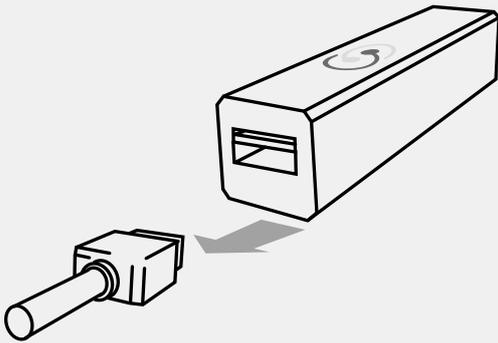
1. Unplug the USB cable from the calibrator unit and remove the USB cable from the power source.
