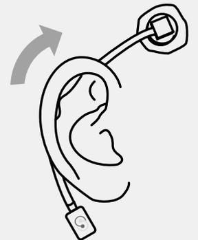
3. After inserting the earplug to be tested in the ear, position the probe with the plastic tube behind the ear. Ensure the plastic tube is pointing upwards to the top part of the helix of the ear.
