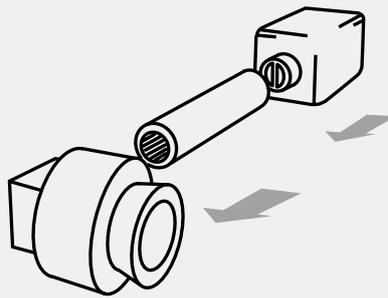
2. Attach the required adaptor that matches the filter of the earplug to be tested at the other end of the plastic tube.
