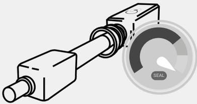
4. Do a test whilst the sealCheck probe is still inserted into the calibrator unit.
