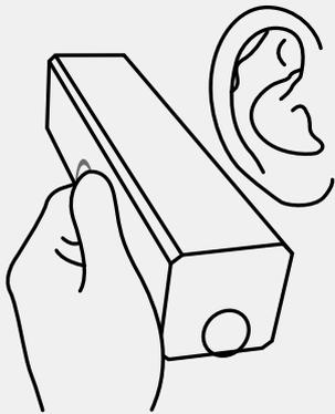
4. Place the calibrator unit close to your ear to listen for noise being generated from the inside of the calibrator unit.
