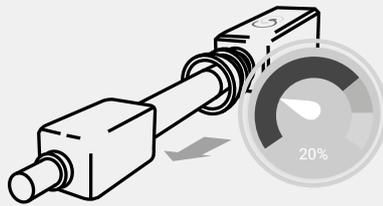
5. When removing the probe from the calibrator make sure that there is a significant drop in the seal indicator.
