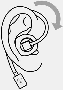
4. Place the plastic tube over the helix towards the ear canal to be attached to the earplug being tested. Attach the adaptor onto the earplug.
