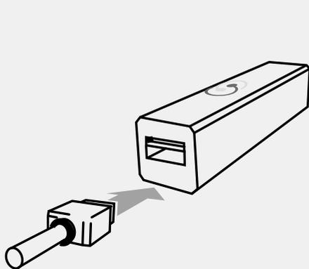
1. Use the supplied USB cable and plug it into the calibrator unit and insert the other end into a power source (i.e. smartphone device charger, computer)
