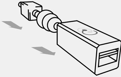
5. Insert the probe assembly into the calibrator unit's opening. Confirm the sealCheck probe has been inserted into the calibrator unit until the probe stopper presses against the calibrator unit. Leave the assembly for a few seconds for the eartip to settle inside the calibrator cavity before starting calibration.
