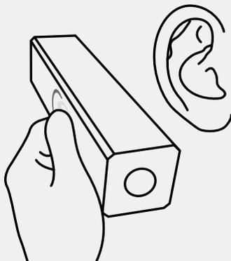
2. Place the calibrator close to your ear to listen if a noise is generated inside the calibrator unit. Confirm this on the sealCheck application. Should no noise be coming from the calibrator unit please revert to the TROUBLESHOOTING section.
