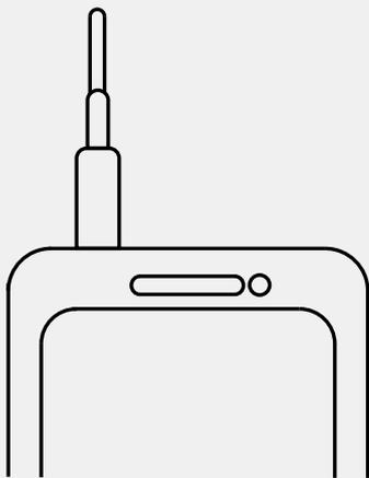
1. Make sure that the audio connector of the sealCheck probe is tightly inserted and makes good contact with the smartphone device.
