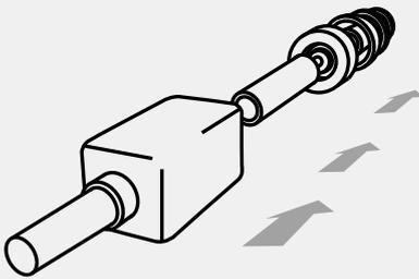
1. Remove the standard three-flange eartip and probe assembly used to complete the calibration process from the sealCheck probe. Do not remove the plastic tube.
