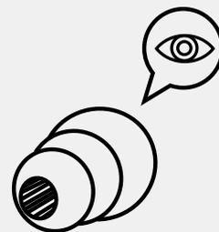
3. Take the provided eartip and ensure there is no obstruction inside before attaching it to the sealCheck probe nozzle.
