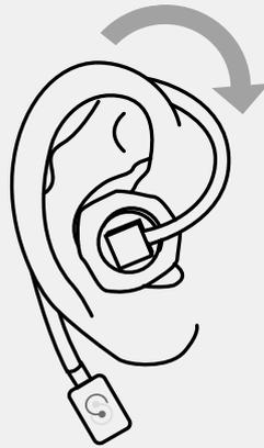
5. Place the plastic tube over the helix towards the ear canal to be attached to the earplug being tested. Attach the adaptor onto the earplug.
