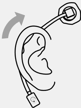
4. After inserting the earplug to be tested in the ear, position the probe with the plastic tube behind the ear. Ensure the plastic tube is pointing upwards to the top part of the helix of the ear.
